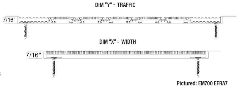
2. Use shims to raise frame to exact height of finished floor and level the frame.
