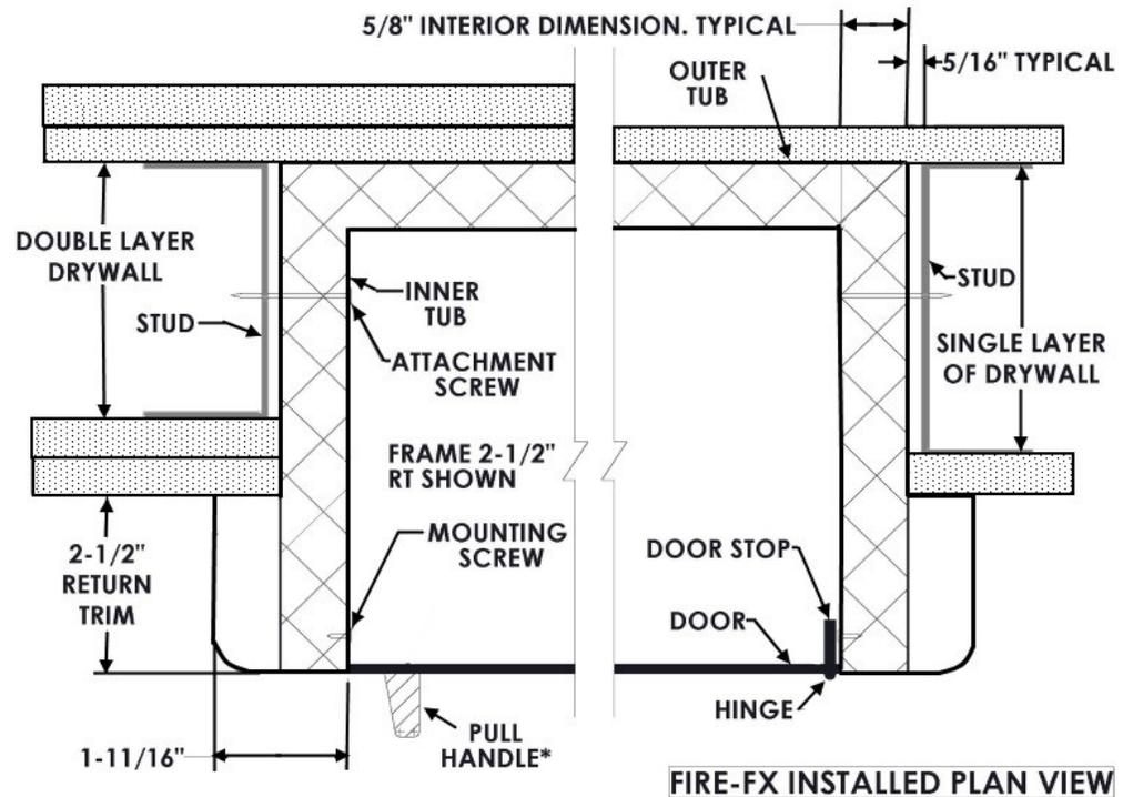
**NOTE:** The installation of any fire-rated cabinet which lacks a cabinet door, or any condition in which the door is left ajar, will void the fire rating
