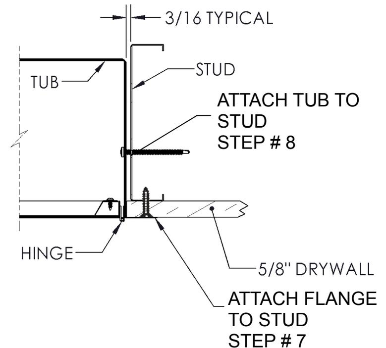
**We Recommend Attaching the Drywall Flange
