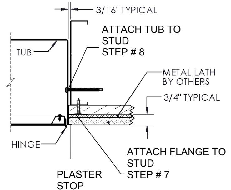
**We Recommend Attaching the Plaster Flange to the Face of the Wall Substrate Before Attaching Tub to the Stud for this Model**
