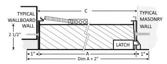
CEILING INSTALLATION (Side View) Use "C" Dimension for Stud to Stud or Masonry Installation Without Wallboard Liner
