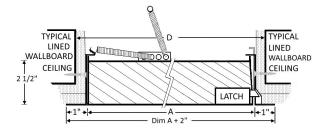
Sizes not shown available upon request up to 48" x 48" in 1/4" increments. Use table on "Made-to-Order" for other sizes. For Sizes Where Height Exceeds 48", See the FCI Series Access Panels
