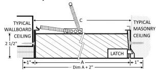
CEILING INSTALLATION (Side View) Use "D" Dimension When Using Wallboard Liner of Opening on 4 Sides
