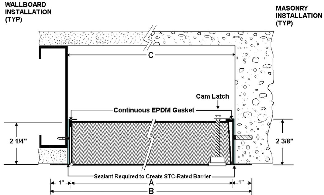
THE STC ACCESS PANEL CAN BE INSTALLED IN A WIDE RANGE OF STC-RATED WALLS
