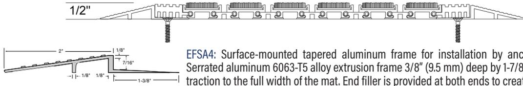
**EFSA4:** Surface-mounted tapered aluminum frame for installation by anchoring to floor. Serrated aluminum 6063-T5 alloy extrusion frame 3/8" (9.5 mm) deep by 1-7/8" (47.6 mm) give traction to the full width of the mat. End filler is provided at both ends to create a snug fit.
