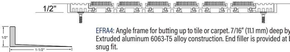
**EFRA4:** Angle frame for butting up to tile or carpet. 7/16" (11.1 mm) deep by 1/8" (3.2mm) profile. Extruded aluminum 6063-T5 alloy construction. End filler is provided at both ends to create a snug fit.
