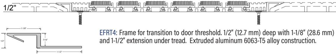
**EFRT4:** Frame for transition to door threshold. 1/2" (12.7 mm) deep with 1-1/8" (28.6 mm) face and 1-1/2" extension under tread. Extruded aluminum 6063-T5 alloy construction.
