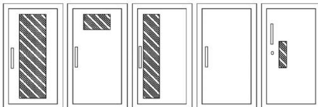
**ADA Cabinet Mounting Height:** Standard Pull on G, E, W, L22 and B Door Styles with Saf-T-Lok are 3 5/8" Higher than Door Center, so Allow for that When Mounting Cabinet.
