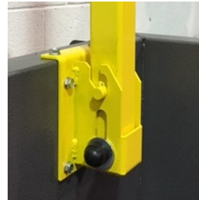
Post Installs to Roof Hatch Curb with 6 Self-tapping Screws
